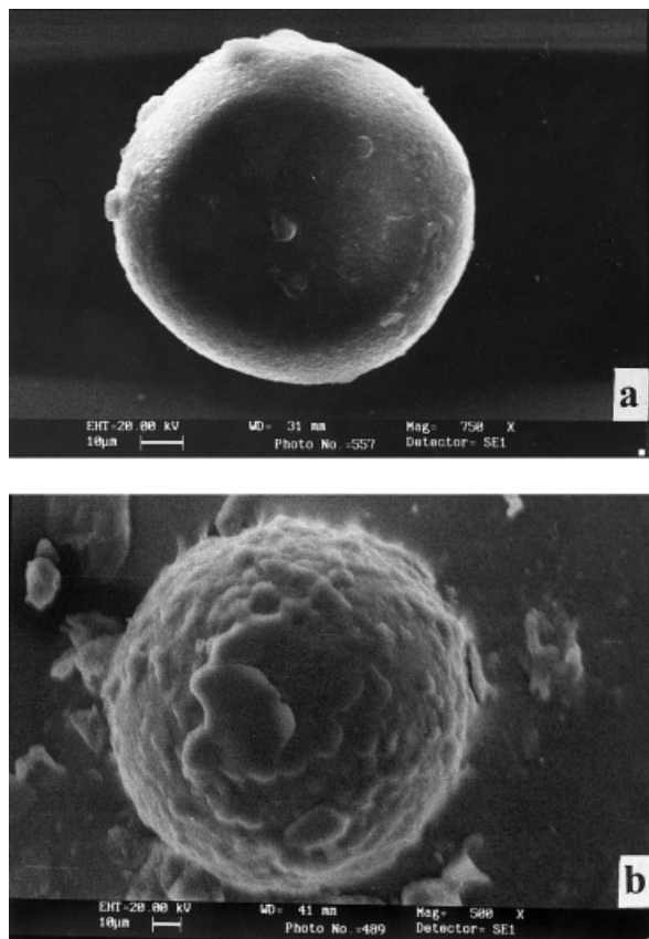
Figure 3 A representative scanning electron micrograph of dried microspheres: (a) PMMA core microspheres; and (b) poly(MMA-HEMA) core-shell hydrogel microspheres.
